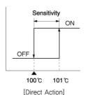
Ex.) In the temperature controller of temperature Ex.) In the temperature controller of temperature range between 0  $\sim$  400 °C, if the set up is 100 °C with the adjustment sensitivity is 1 °C, it is Off at 100 °C and On at 101 °C.
