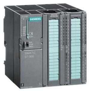
SIMATIC S7-300, CPU 313C, CPU COMPACTA CON MPI, 24 ED/16 SD, 4EA, 2SA, 1 PT100, 3 CONTADORES RAPIDOS (30 KHZ), FUENTE ALIM. INTEGRADA 24V DC, MEMORIA CENTRAL 128 KBYTE, REQUIERE CONECTOR FRONTAL (1X 40 POLOS) Y MICRO MEMORY CARD
