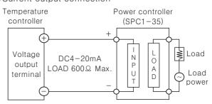
$\Re$  The current value of DC4−20mA is available at lower than 600 Ω of resistive load.
