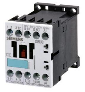
CONTACTOR, AC-3 4 KW/400 V, 1 NO, AC 110 V, 50/60 HZ, 3-POLE, SIZE S00, SCREW CONNECTION
