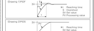
There are high-speed response type and low-speed response type built in this unit. Therefore user can select each function according to their application
