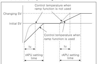
It makes delay rising temperature when change the set value at stable control status or delay the initial rising temperature as above picture.
