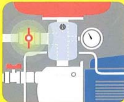
1) CLOSE THE DELIVERY SIDE OF THE SYSTEM
